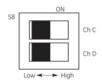
If a low audio level causes the output audio signal to degrade, the input sensitivity of the A8920A can be increased by switching to the 8 dBu maximum scale.
